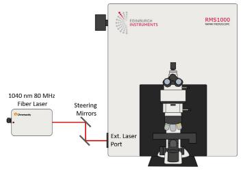
**FIGURE 1.** Schematic of the second harmonic process. This nonlinear optical process, causes two long wavelength photons to interact within a material to form new photons having twice the frequency of the input photons.
